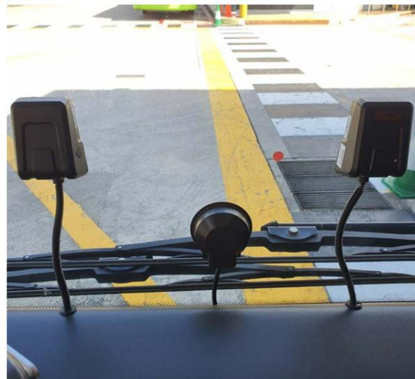
Smart Advanced Warning Unit sensors provide bus drivers with advanced pedestrian and vehicle collision alerts.
