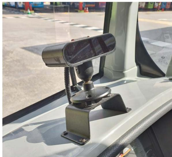
Seeing Machines Guardian's Driver Alert Camera (T-DA) system provides fatigue detection and alerts with incident reporting capability.
