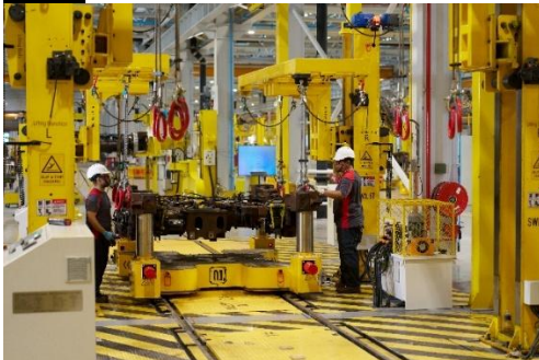
Photo of the Rail Guided Vehicle delivering a bogie frame to the Bogie Assembly Equipment.
