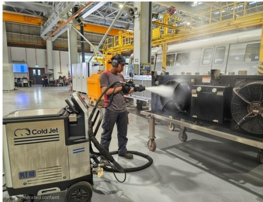
Photo of staff using dry ice cleaning machine to remove dirt from a train component
