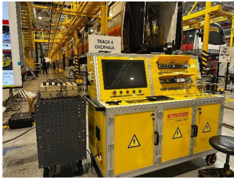
Photo of Relay Test Bench
