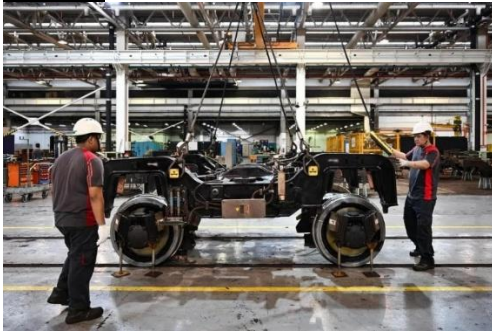
Photo of staff lowering a bogie frame onto the wheelsets using overhead crane.
