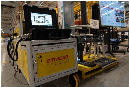
Photos of Master Controller Test Bench
