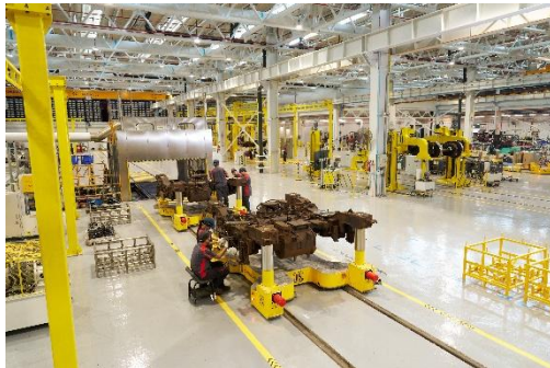
Photo of a maintenance staff working on a bogie frame transported on a yellow Rail Guided Vehicle
