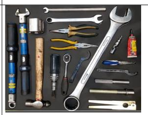
Tools are now neatly arranged in a tools template, which is a foam cut-out crafted by our staff. Each workbench is assigned a tools template. From a glance, our staff are able to tell if any tools are missing, reducing time wastage in locating the tools. Apart from the tools template, workbenches are now tagged with names of workers, strengthening their sense of ownership and accountability for each piece of equipment and for the cleanliness of their workbench at the end of a work day.
