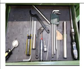
Work bench tools were not sorted according to how frequently such tools were used. This caused inefficiency as time may be wasted to search for tools while technicians are carrying out their work.
