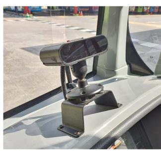
Seeing Machines Guardian's Driver Alert Camera (T-DA) system provides fatigue detection and alerts with incident reporting capability.
