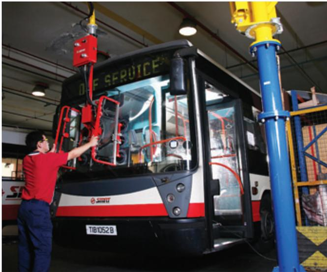
Several bus upgrading and improvement projects are currently underway to improve the reliability and safety of our buses. These include air system enhancement (Dennis buses), floorboard replacement (Mercedes buses), LED electronic destination system upgrading, as well as bus air-condition evaporator/condenser coil replacement.
